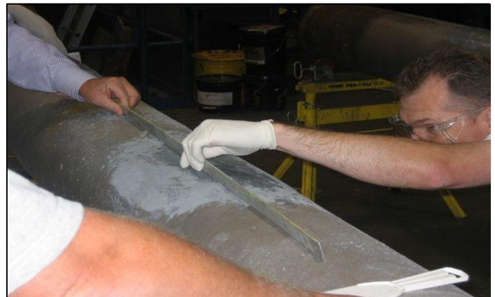
Fig. 5 – Use a ruler to confirm the uniformity of the filler putty
